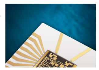
being held in Atlanta, GA, from June 8-9. StratEdge packages operate from DC to 63+ GHz and dissipate heat from compound semiconductor devices such as gallium nitride (GaN), gallium arsenide (GaAs), and silicon carbide (SiC). These packages enable compound semiconductor devices to meet the critical requirements of markets such as telecom, mixed signal, VSAT, broadband wireless, satellite, military, test and measurement, automotive, and down-hole.
